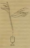
intended to pour. When, by further motion of the vessel, the fluid at last runs over its edge, it will proceed down the rod, being conducted by it in any required direction. When a sufficient quantity has in this way been removed, the vessel is to be restored to its first position, the rod not being withdrawn until the fluid is decidedly below the inside edge; all that is without will be confined to the surface of the rod, not a particle having flowed down the outside of
